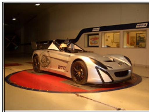
We also took the opportunity to optimise the location and angle of incidence for both the standard and optional wings and the front splitters, giving us an excellent downforce balance for the non-adjustable standard setup and a useful range of complementary settings for the optional adjustable wings.
